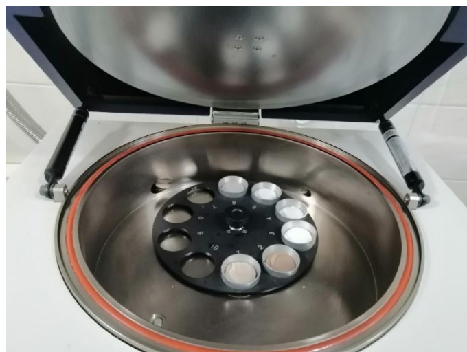
Fig. 5: XRF illustrates the sample chamber.
