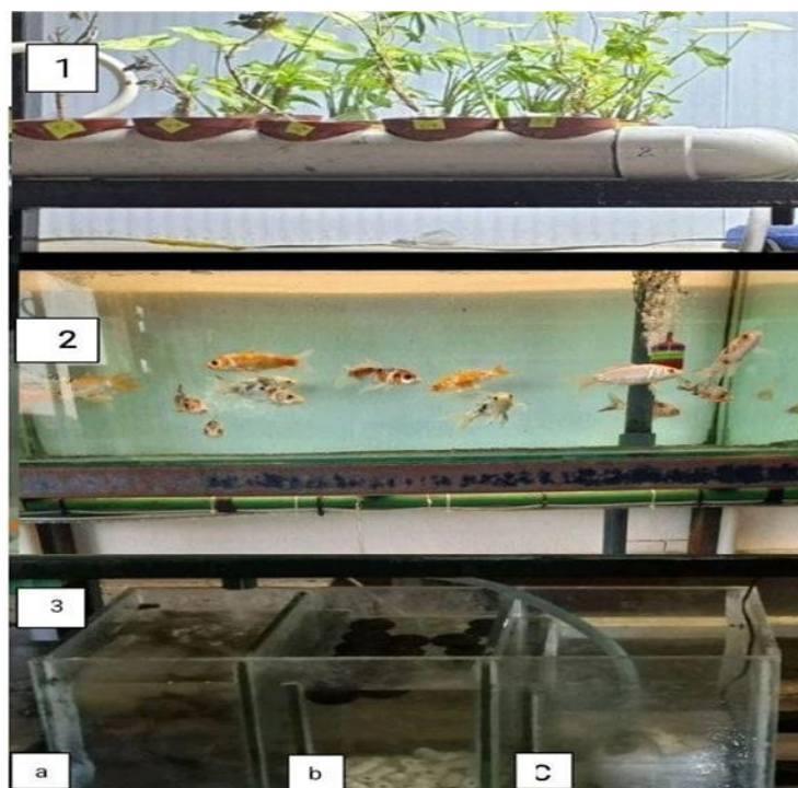
Figure (1): Components of an aquaponic system: (1) Plant culture tubes, (2) Fish culture tanks, (3) Mechanical and biological filter tanks, (a) Mechanical filter, (b) Bio filter, and (c) Water sublimation pump
